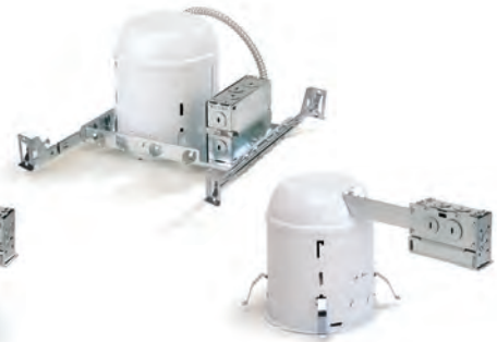
6" Non-IC Line Voltage Housings NH-260 New Construction / 150W max. NH-260NB NB Floating Socket / 150W max. Width: 7" Length: 10-1/8" Height: 7-1/2" NHR-260 Remodel / 150W max. Width: 6-3/4" Length: 13-3/4" Height: 7-1/2"
