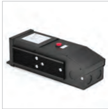
Class II Hardwire LED Driver with Regulator, MLV dimming NMTD-60/24D 60W NMTD-96/24D 96W Voltage: 120-277V/24V Wattage: 60W or 96W Dimming: Magnetic Low Voltage Regulator: Integral regulator for constant current and voltage Includes: 10' Power Line Connector
