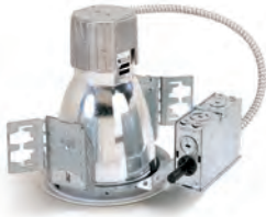
6" Architectural Line Voltage Frame-In NHAV-6150 150W A21 / PAR38 Width: 11-3/8" Length: 12" Height: 10-1/2"
