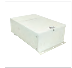
Class II Hardwire LED Driver with Breakers, MLV dimming NMT-303/24C2D1 120V NMT-303/24C2D2 277V Voltage: 120V or 277V/24V Wattage: (3) 100W Dimming: Magnetic Low Voltage Includes: (3) 10' Power Line Connectors
